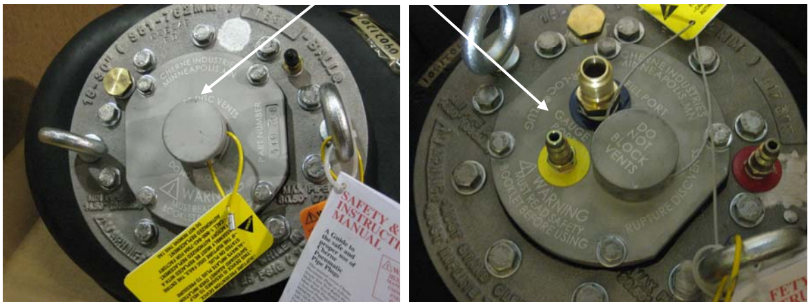
Figure A1 Test-Ball® (Left) and Air-Loc® (Right) with Center Plate Housing RPD
